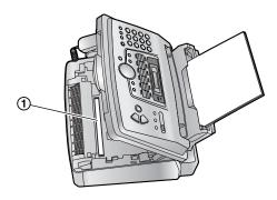
**9** Reinstall the drum and toner unit (1) by holding the tabs.
